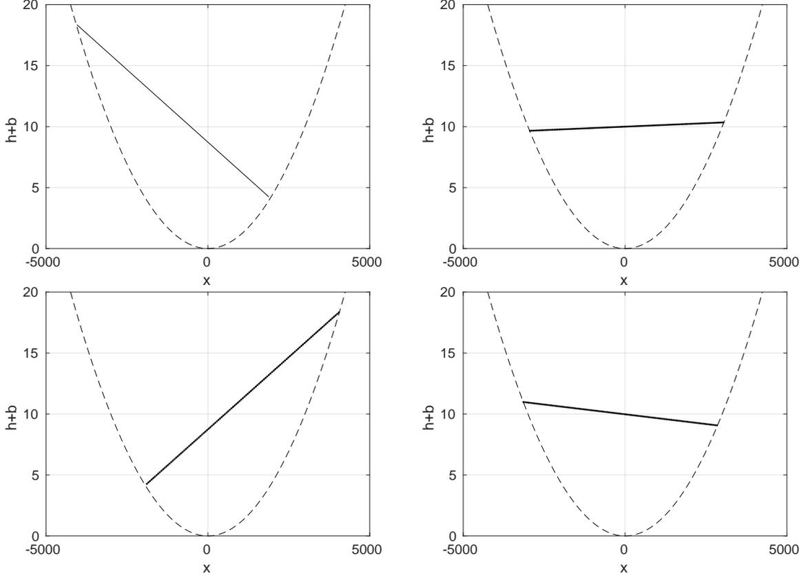
Figure 3. Snapshots of the numerical solution (solid line) and analytical solution (dotted line) of the surface elevation for the parabolic bowl bathymetry (dashed line) at times  $t = 0$ ,  $t = 1000$ ,  $t = 2000$  and  $t = 3000$ .
