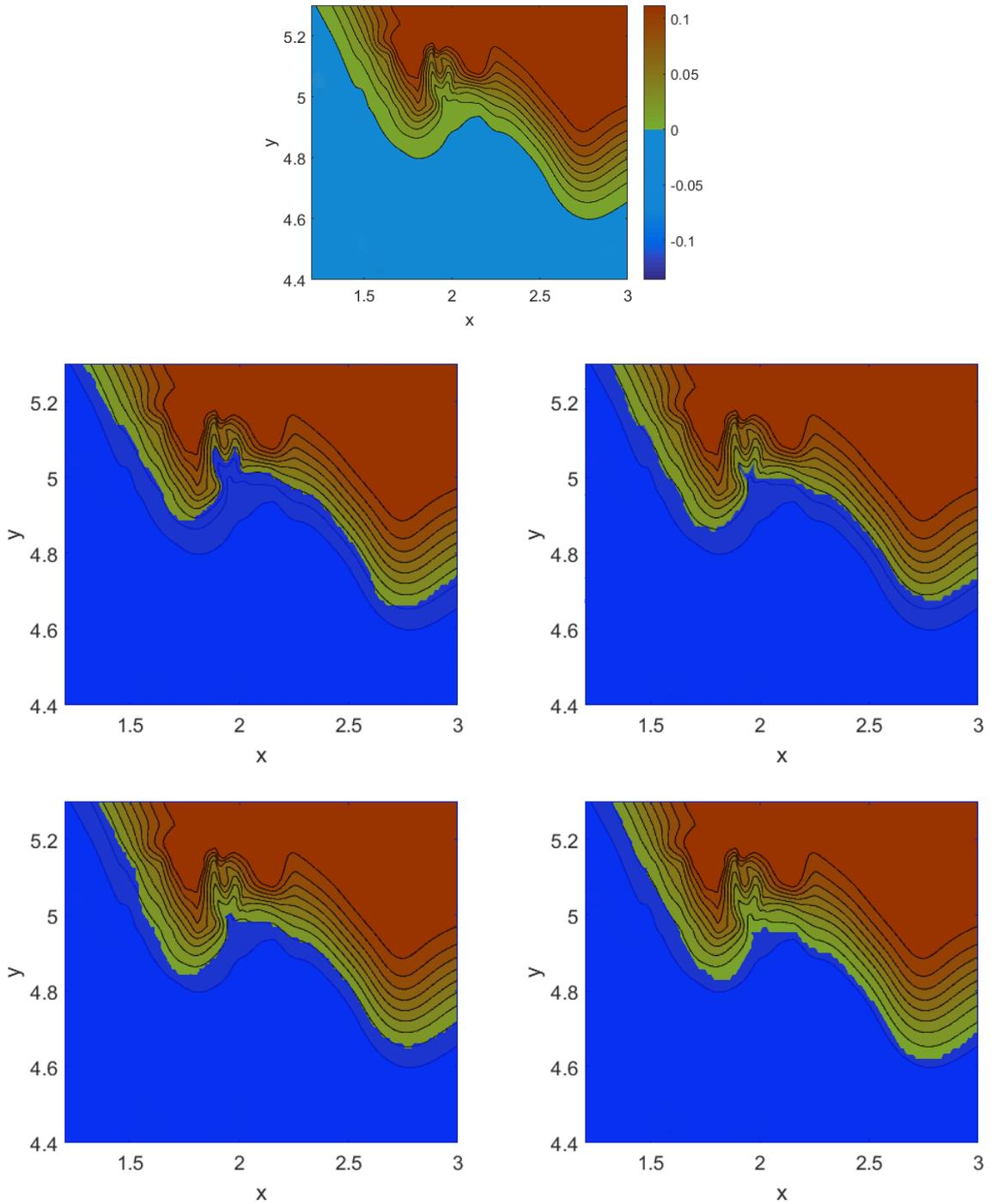
Figure 12. Image at the top shows the initial water elevation and the height of the valley. Snapshots of the computed solution ( $h + b$ ) for the Monai Valley test case at times  $t = 16.2$  (top left) (time of maximal run-up),  $t = 17$  (top right),  $t = 18$  (lower left) and  $t = 19$  (lower right).
