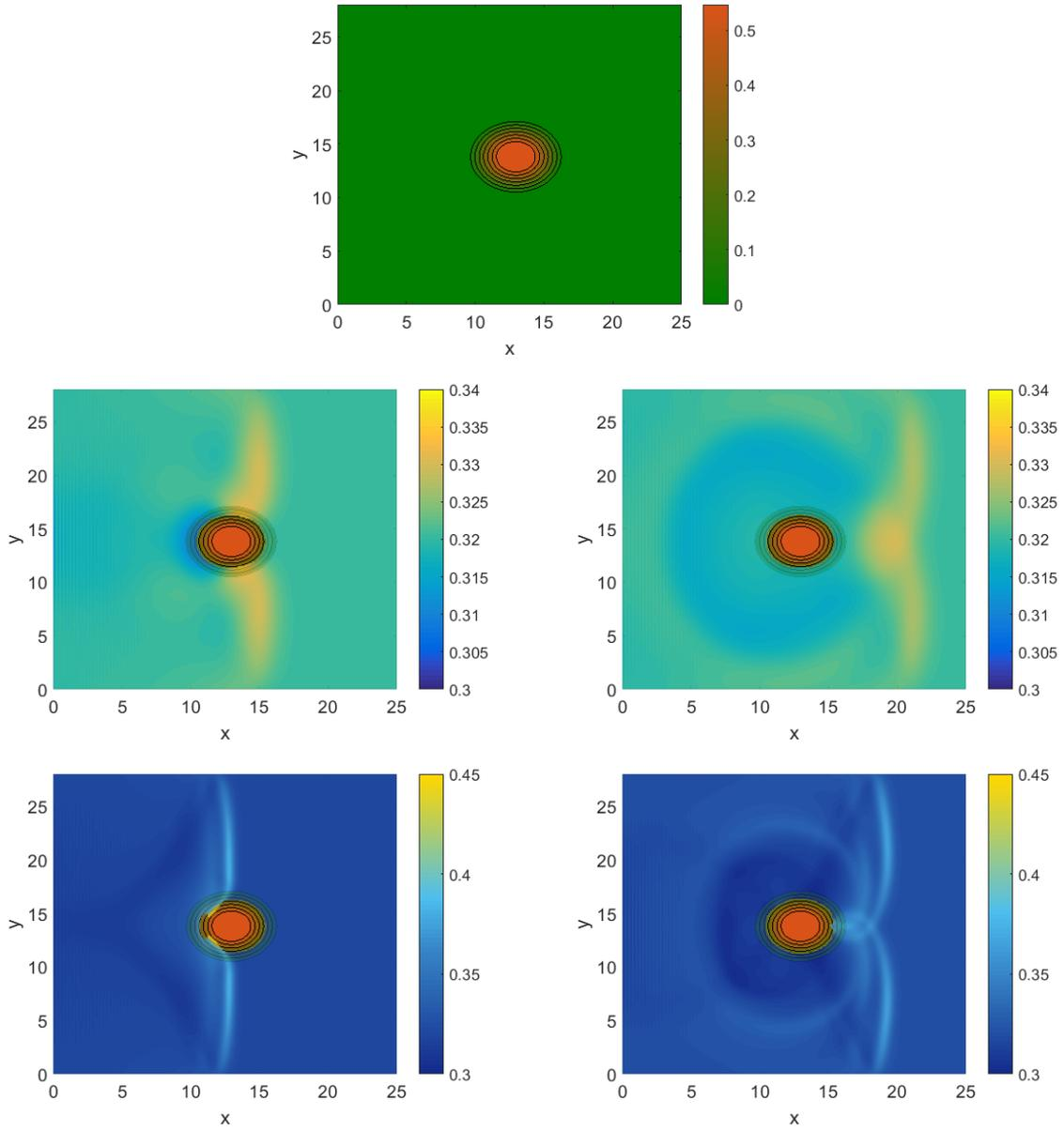
Figure 10. Image at the top shows the initial water elevation and the height of the island. Snapshots of the computed solution  $(h + b)$  for the conical island test case at times  $t = 12$  and  $t = 16$  for case A (above) and at times  $t = 10$  and  $t = 14$  for case C (below) for the conical island.
