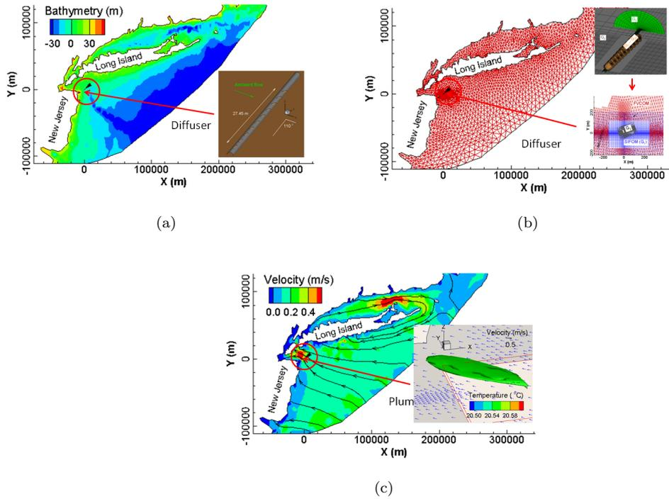
Fig. 10: Simulation of thermal discharge from the bottom of the ocean, obtained with the SIFOM-FVCOM [342]. (a) Computational domain and bathymetry. (b) Grids. (c) Simulated instantaneous flow field and thermal plume. The red lines indicate the interface between SIFOM and FVCOM.
