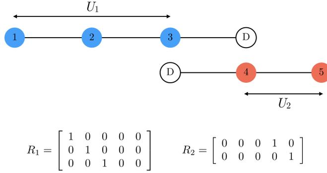
Fig. 3: The multiplicative Schwarz method (a block Gauss-Seidel method) with a minimum overlap. Nodes applied with Dirichlet conditions are indicated with a D.
