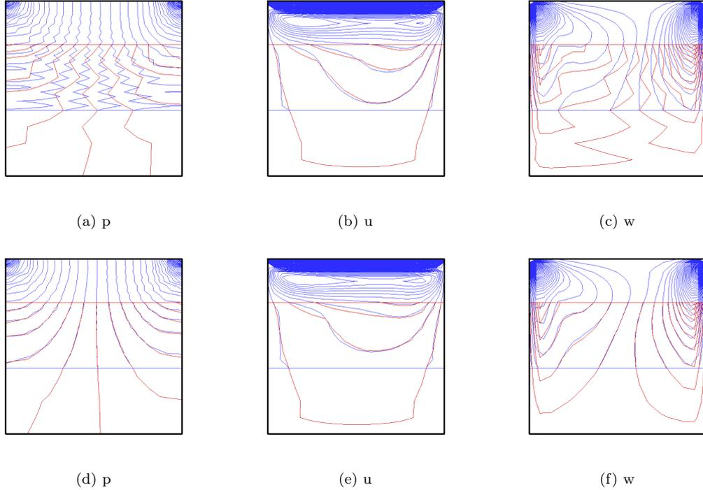
Fig. 9: Simulation of a 3D oscillating cavity flow at  $t = 10$  with  $Re = 100$  [338].  $p$  is pressure, and  $u$  and  $v$  are velocity in the horizontal and vertical direction, respectively. Two overlapping grids are used and arranged vertically. (a), (b), (c) Solutions obtained with interpolation at the grid interfaces. (d), (e), (f) Solutions obtained with MFBI at the grid interfaces.
