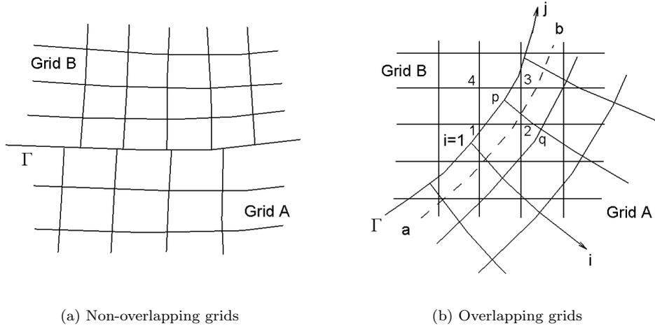
Fig. 6: Typical layouts of grids in simulation of fluids.
