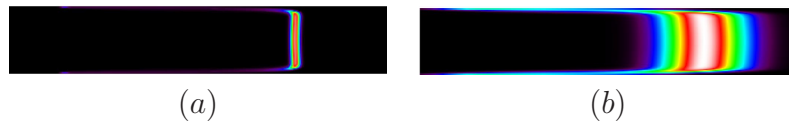
Figure 2: Comparison of a fully-Lagrangian parcel advection method with a flux-form Eulerian scheme. The error accumulates drastically in the Eulerian scheme. The concentration of an invading fluid injected into a confined channel containing a resident fluid is predicted at finite time t : (a) Parcel advection method, (b) Flux-form Eulerian scheme.
