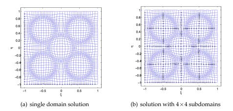
Figure 2: A comparison of the single domain mesh and the mesh obtained for  $4\times4$  subdomains for the five ring problem.
