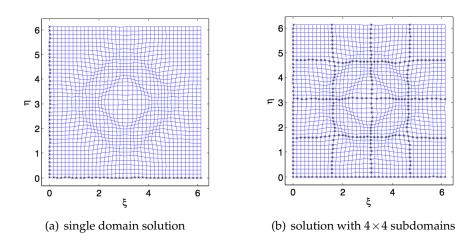
Figure 3: A comparison of the single domain solution and that obtained for  $4\times4$  subdomains for the shallow water equations at t=0.15.
