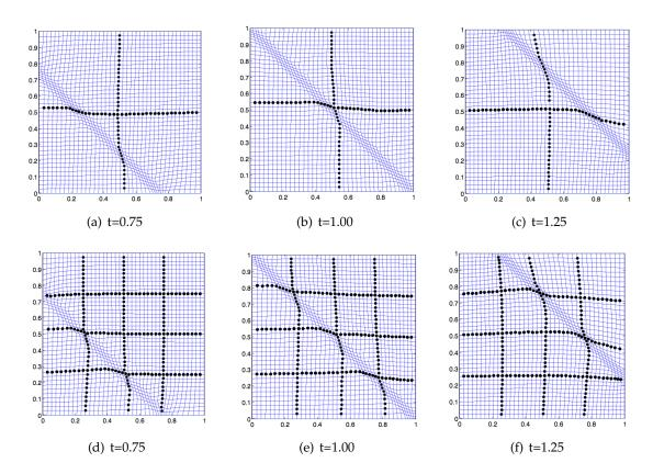
Figure 1: Evolution of mesh for Burgers' equation using the stochastic DD method with  $2\times 2$  (top) and  $4\times 4$  (bottom) subdomains.
