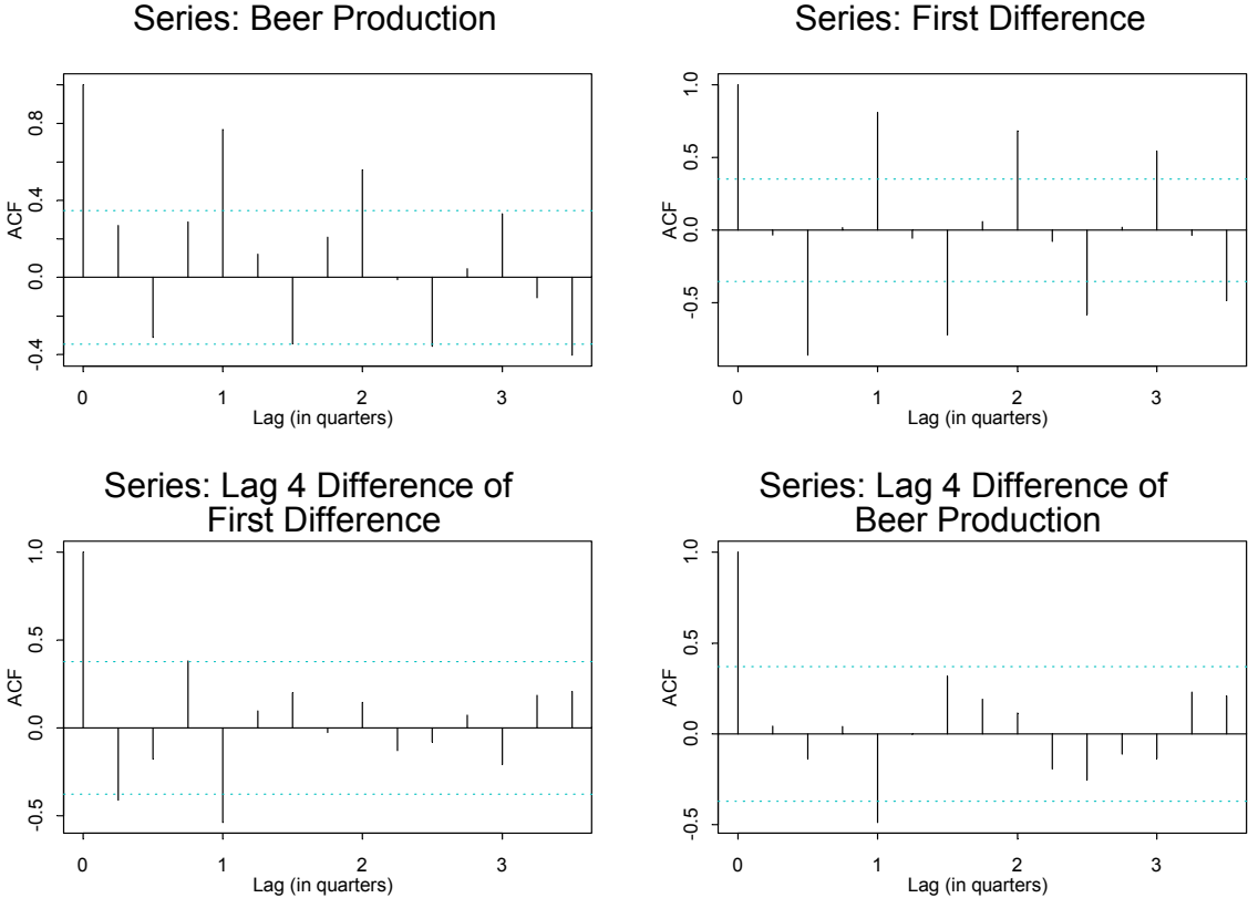
Figure 18: Plot of the sample autocorrelation function for: (a) beer production series (b) first difference of beer series (c) lag 4 difference of the first difference (d) lag 4 difference of the beer series.
